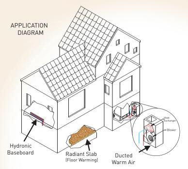
With the optional air handler, you can enjoy forced air heating and/or cooling in addition to radiant hydronic heating.
